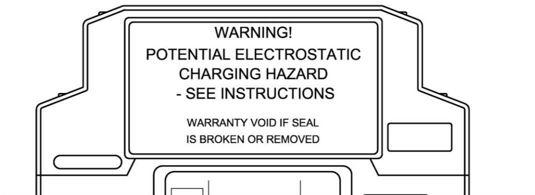
Figure 2. Warning plate - protective seal.
