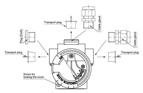
Figure 1. 10. Installation of cable entries and blinding plugs (example).
