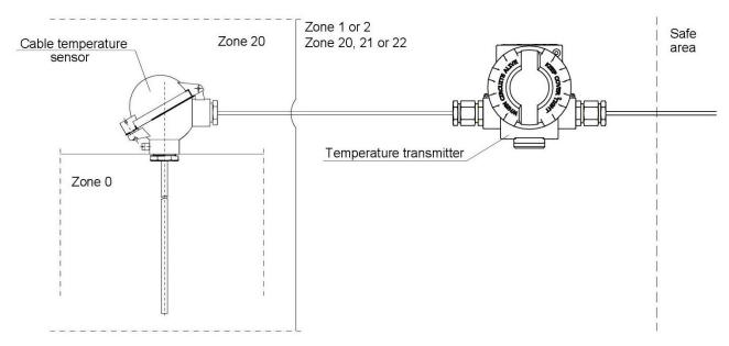
Figure 1. 3. LI-24ALW temperature transmitter with a cable temperature sensor.
