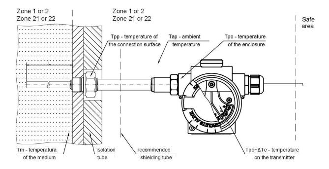
Figure 2. 6. Determination of the temperature of transmitter with sensor screwed into the enclosure.
