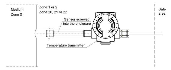
Figure 1. 4. LI-24ALW temperature transmitter with a sensor screwed into the enclosure.
