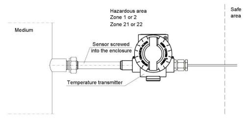
Figure 2. 4. LI-24ALW temperature transmitter with a sensor screwed into the enclosure.
