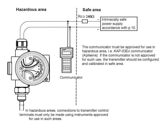
Figure 1. 9. Connection of the transmitter in Exi version.
