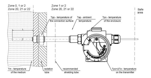
Figure 1. 8. Determining the working temperature of the transmitter.
