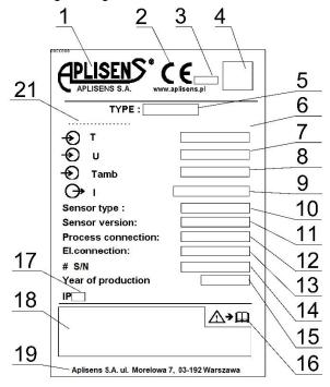
Figure 1. 1. Example of a nameplate for a transmitter with a direct sensor.
