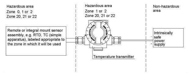
Figure 1. 5. Temperature transmitter with a cable temperature sensor or with a sensor screwed into the enclosure.
