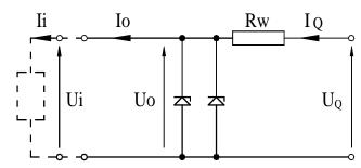
Figure 1.7. The principle of power supply from a source with a trapezoidal characteristic.
